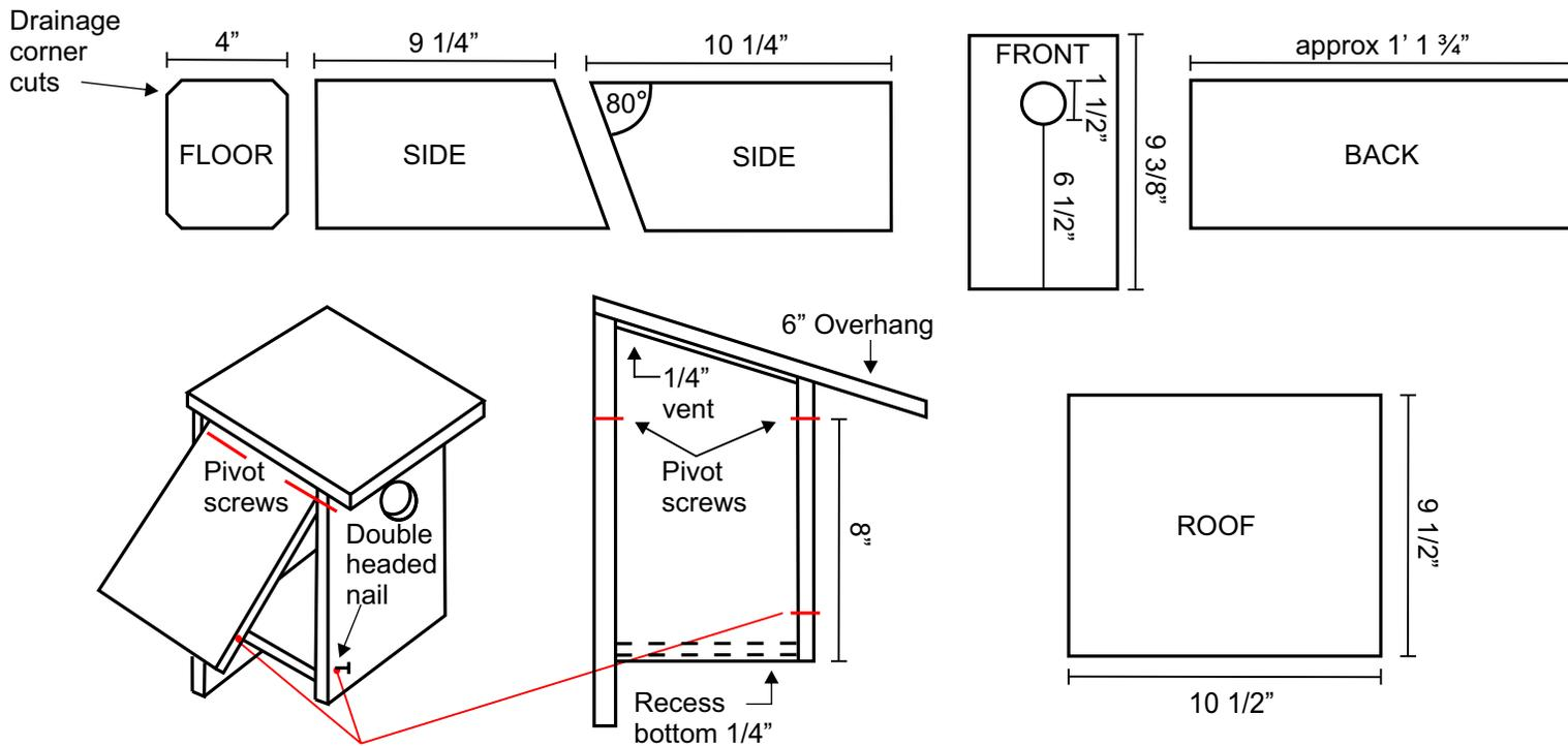
Drill hole through "front" and side of door to hold door closed with nail.
